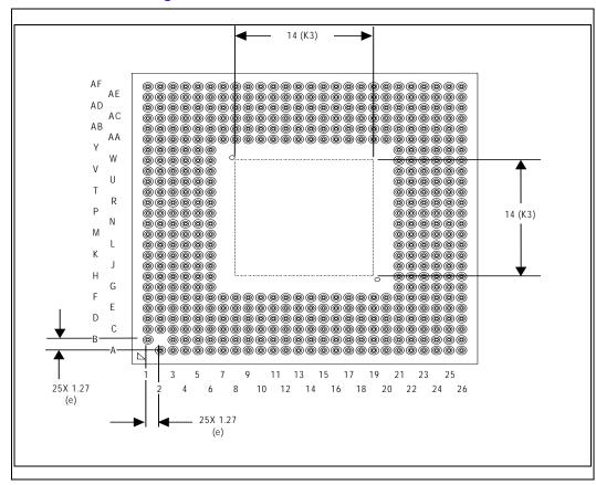
Figure 4-3. Micro-FCPGA Package - Bottom View
