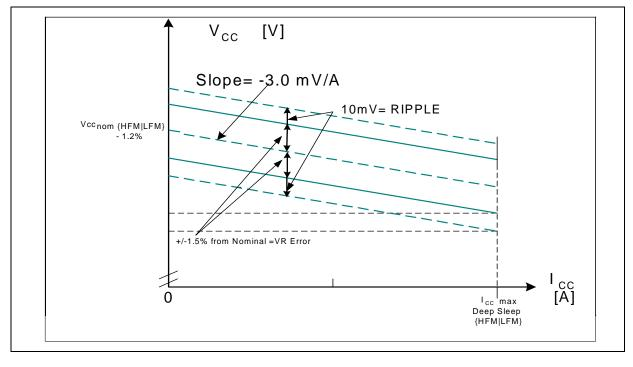
Figure 3-2. Deep Sleep VCC and ICC Load Line
