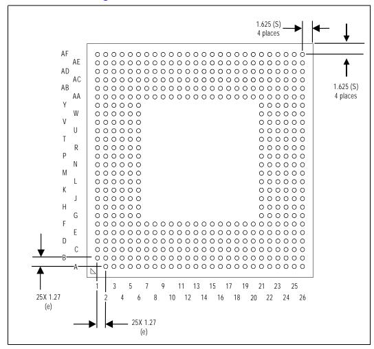
NOTE: All dimensions in millimeters. Values shown for reference only. Refer to Table 4-2 for details.
