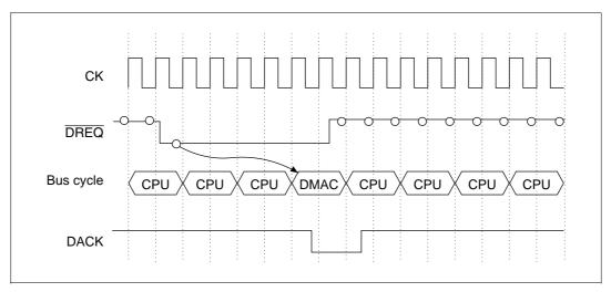
Figure 9.15  $\overline{DREQ}$  Sampling Timing in Cycle Steal Mode (Output with  $\overline{DREQ}$  level detection and DACK active low) (Single address mode, bus cycle = 2 states)
