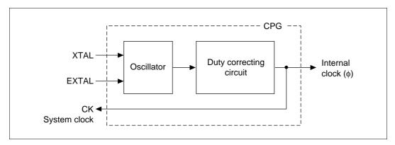
Figure 7.1 Block Diagram of the Clock Pulse Generator
