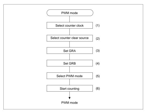
Figure 10.28 Procedure for Selecting the PWM Mode
