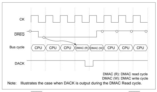
Figure 9.14  $\overline{DREQ}$  Sampling Timing in Cycle Steal Mode (Output with  $\overline{DREQ}$  level detection and DACK active low) (Dual address mode, bus cycle = 1 state)
