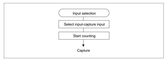
Figure 10.23 Procedure for Selecting Input Capture Mode
