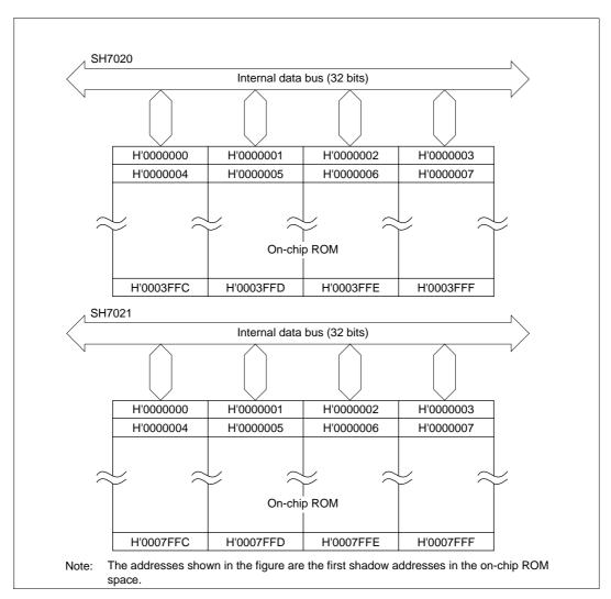
Figure 16.1 Block Diagram of ROM
