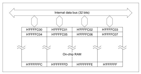
Figure 17.1 Block Diagram of RAM
