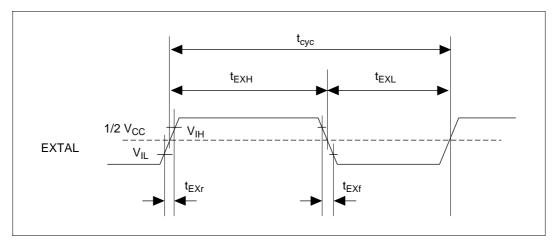
Figure 19.1 EXTAL Input Timing
