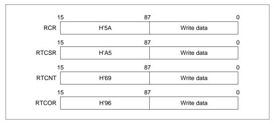
Figure 8.2 Writing to RCR, RTCSR, RTCNT, and RTCOR
