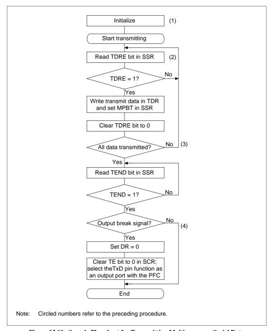
Figure 13.10 Sample Flowchart for Transmitting Multiprocessor Serial Data
