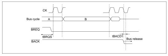
Figure 8.43 When BREQ is Input without Satisfying tBRQS
