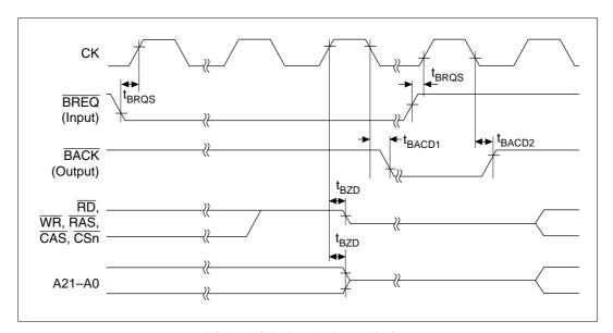
Figure 19.7 Bus Release Timing
