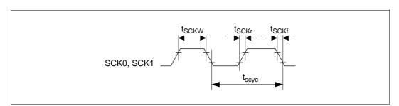
Figure 19.40 Input Clock Timing
