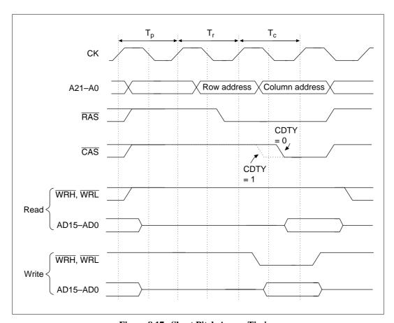
Figure 8.17 Short Pitch Access Timing
