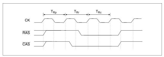
Figure 8.30 Output Timing for CAS-Before-RAS Refresh Signal
