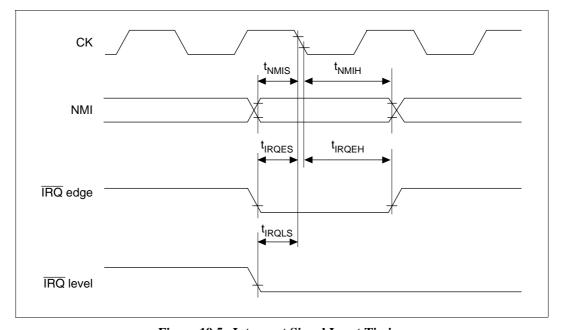
Figure 19.5 Interrupt Signal Input Timing
