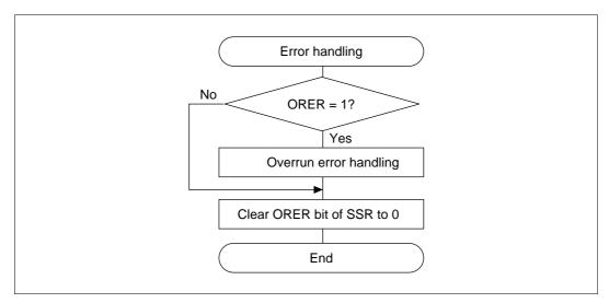
Figure 13.18 Sample Flowchart for Serial Receiving (cont)
