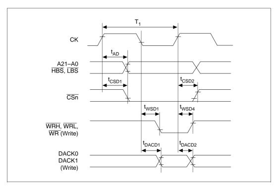
Figure 19.33 DMA Single Transfer/Single State Access Write
