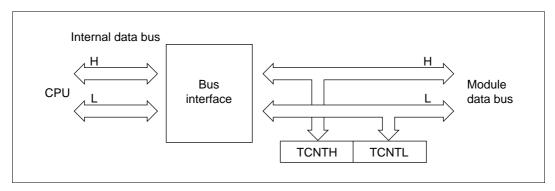
Figure 10.9 Accessing TCNT (CPU-TCNT (lower byte))
