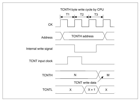
Figure 10.60 Contention between TCNT Byte Write and Increment
