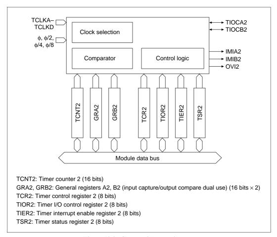
Figure 10.3 Channel 2 Block Diagram
