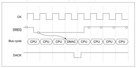
Figure 9.13  $\overline{DREQ}$  Sampling Timing in Cycle Steal Mode (Output with  $\overline{DREQ}$  level detection and DACK active low) (Single address mode, bus cycle = 1 state)
