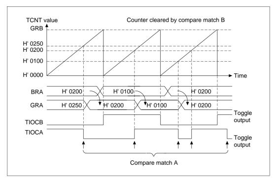
Figure 10.48 Buffer Mode Operation Example 1 (Output Compare Register)
