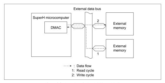
Figure 9.8 Data Flow in Dual Address Mode
