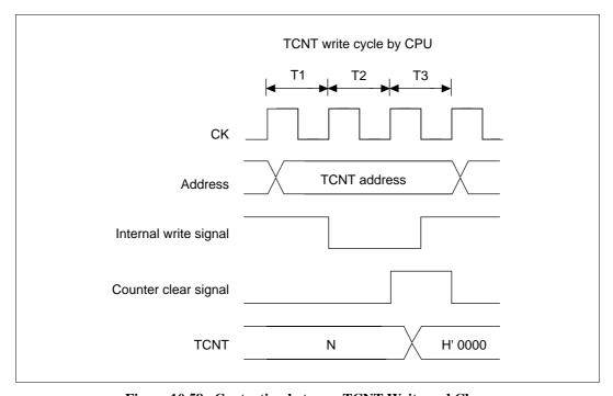
Figure 10.58 Contention between TCNT Write and Clear
