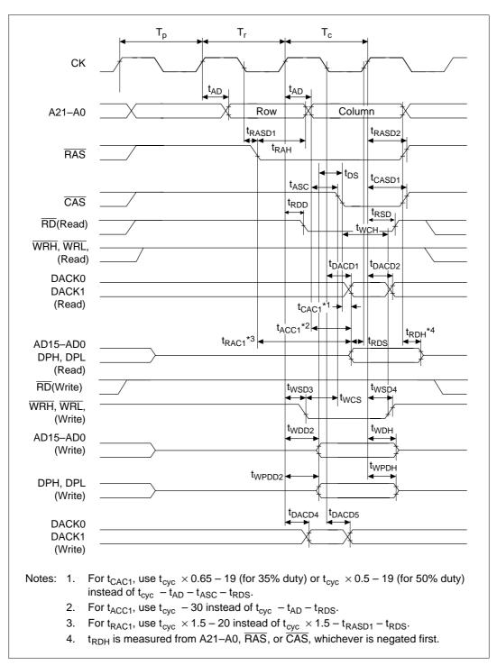
Figure 19.11 DRAM Bus Cycle (Short Pitch, Normal Mode)
