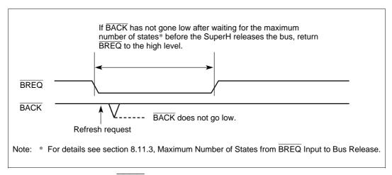
Figure 8.37 BACK Operation in Response to Refresh Request (2)
