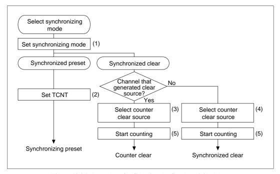
Figure 10.26 Procedure for Selecting the Synchronizing Mode
