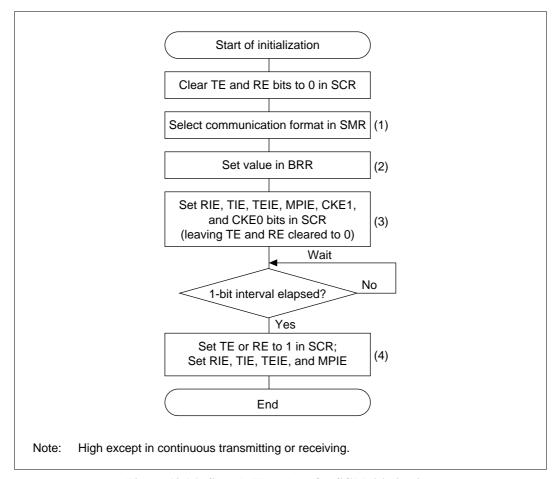
Figure 13.16 Sample Flowchart for SCI Initialization
