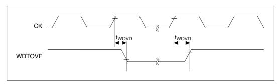
Figure 19.39 Watchdog Timer Output Timing
