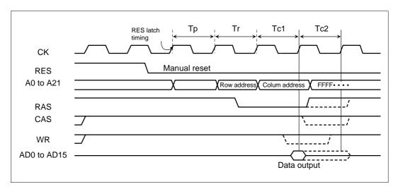
Figure 8.38 Long - pitch Mode Write (1)
