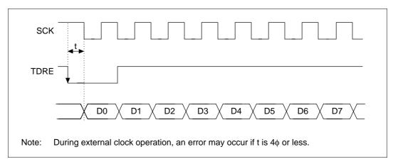
Figure 13.22 Clocked Synchronous Transmitting Example with DMAC
