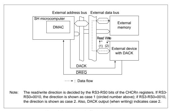
Figure 9.6 Data Flow in Single Address Mode
