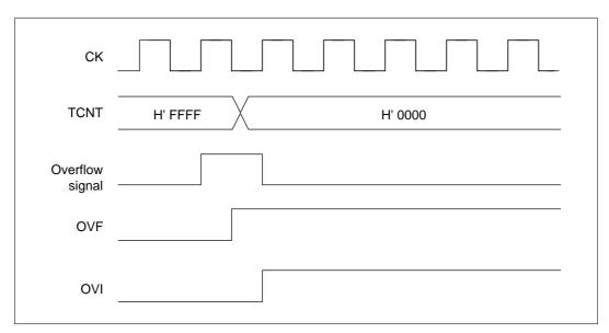
Figure 10.56 Timing of Setting OVF
