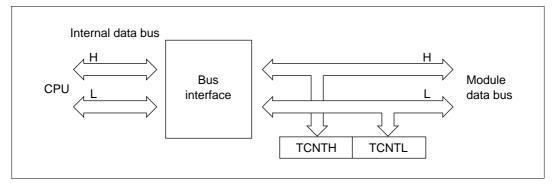
Figure 10.8 Accessing TCNT (CPU-TCNT (upper byte))
