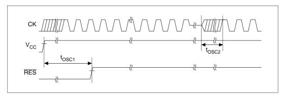
Figure 19.3 Oscillation Settling Time
