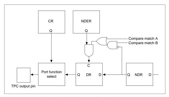
Figure 11.9 TPC Output Non-Overlap Operation
