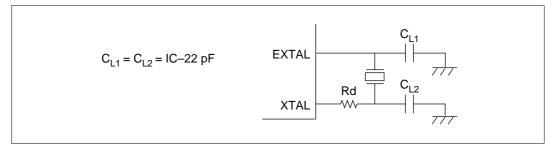
Figure 7.2 Connection of the Crystal Resonator (Example)
