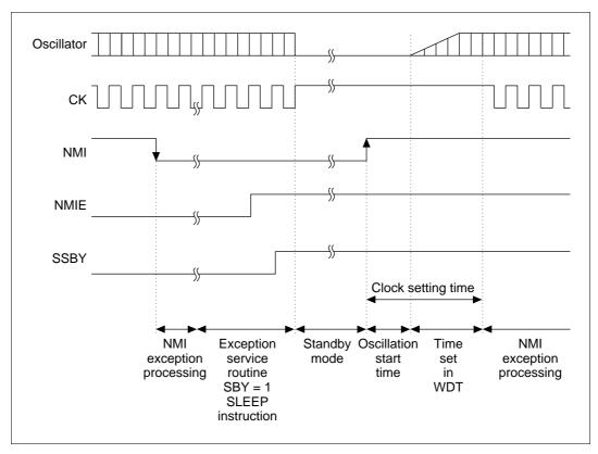
Figure 18.1 NMI Timing for the Standby Mode (Example)
