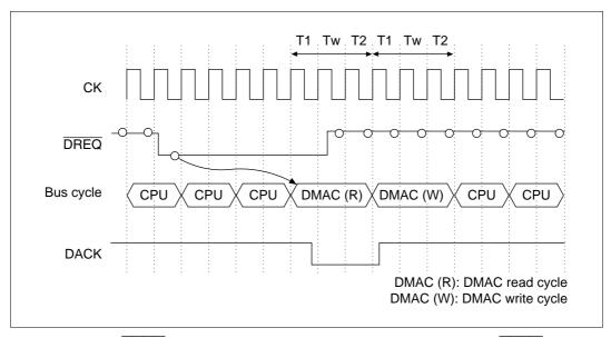
Figure 9.18  $\overline{DREQ}$  Sampling Timing in Cycle Steal Mode (Output with  $\overline{DREQ}$  level detection and DACK active low) (Dual address mode, bus cycle = 2 states + 1 wait state)
