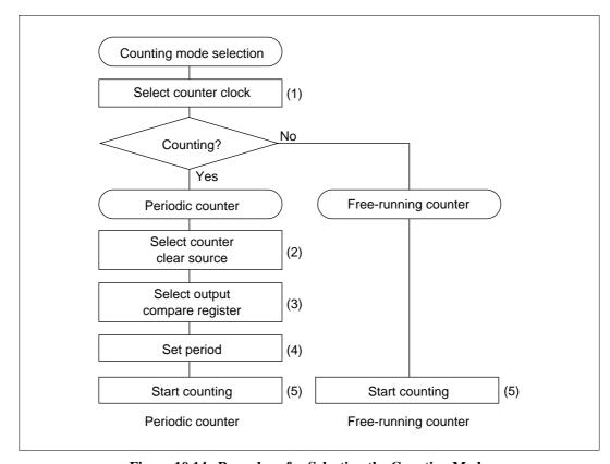
Figure 10.14 Procedure for Selecting the Counting Mode
