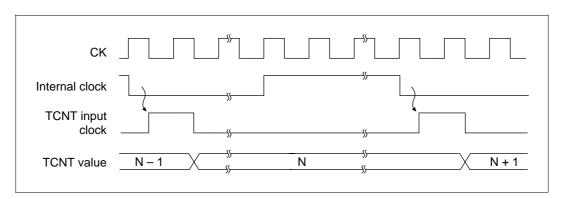
Figure 10.17 Count Timing for Internal Clock Sources
