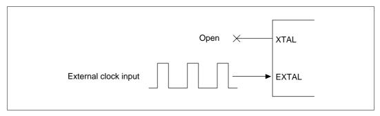
Figure 7.4 External Clock Input Method
