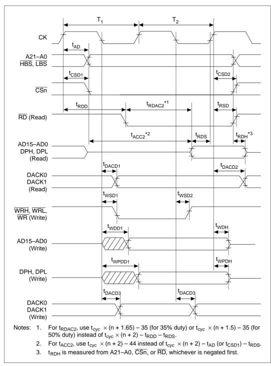
Figure 19.22 Basic Bus Cycle: Two-State Access
