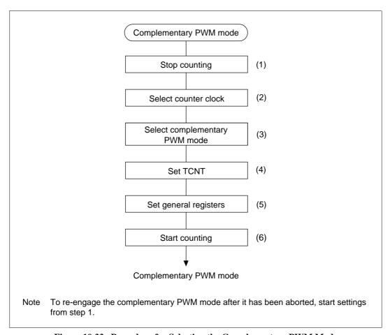
Figure 10.33 Procedure for Selecting the Complementary PWM Mode
