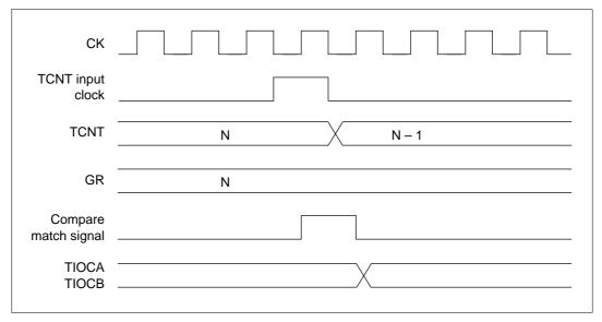
Figure 10.22 Compare Match Signal Output Timing
