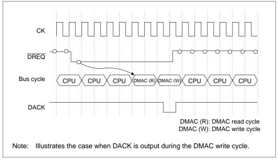
Figure 9.16  $\overline{DREQ}$  Sampling Timing in Cycle Steal Mode (Output with  $\overline{DREQ}$  level detection and DACK active low) (Dual address mode, bus cycle = 2 states)
