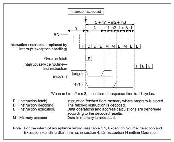
Figure 5.4 Example of Pipelining in IRQ Interrupt Acceptance
