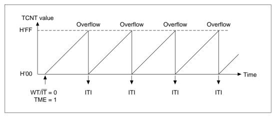
Figure 12.5 Operation in the Interval Timer Mode
