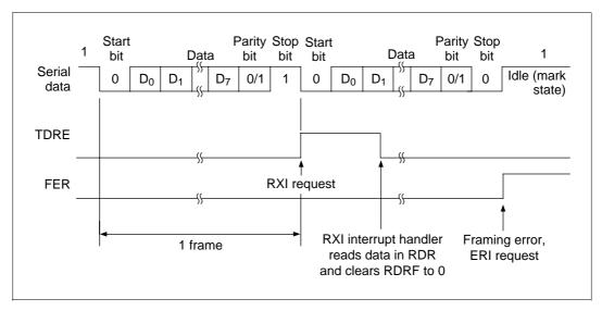
Figure 13.8 Example of SCI Receive Operation (8-bit data with parity and one stop bit)
