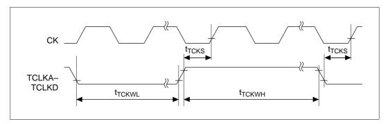
Figure 19.37 ITU Clock Input Timing
