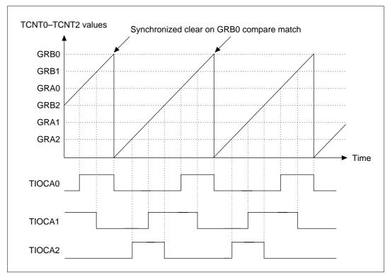
Figure 10.27 Synchronized Operation Example
