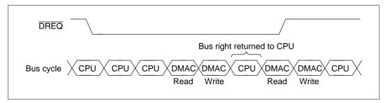
Figure 9.10 Transfer Example in the Cycle-Steal Mode (Dual address mode, DREQ level detection)
