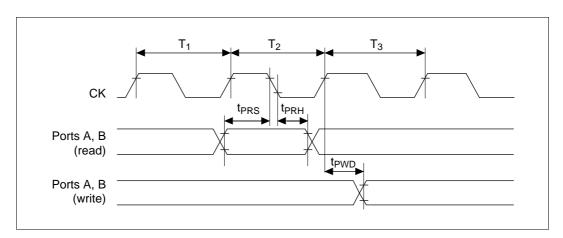
Figure 19.38 Programmable Timing Pattern Controller Output Timing
