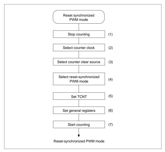
Figure 10.31 Procedure for Selecting the Reset-Synchronized PWM Mode
