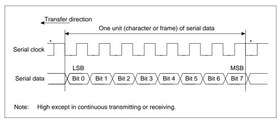
Figure 13.14 Data Format in Clocked Synchronous Communication
