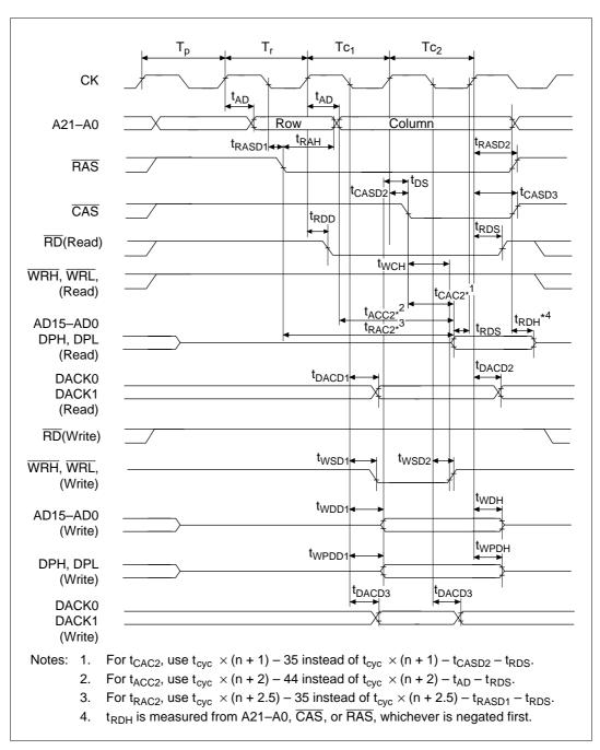
Figure 19.26 DRAM Bus Cycle: (Long Pitch, Normal Mode)
