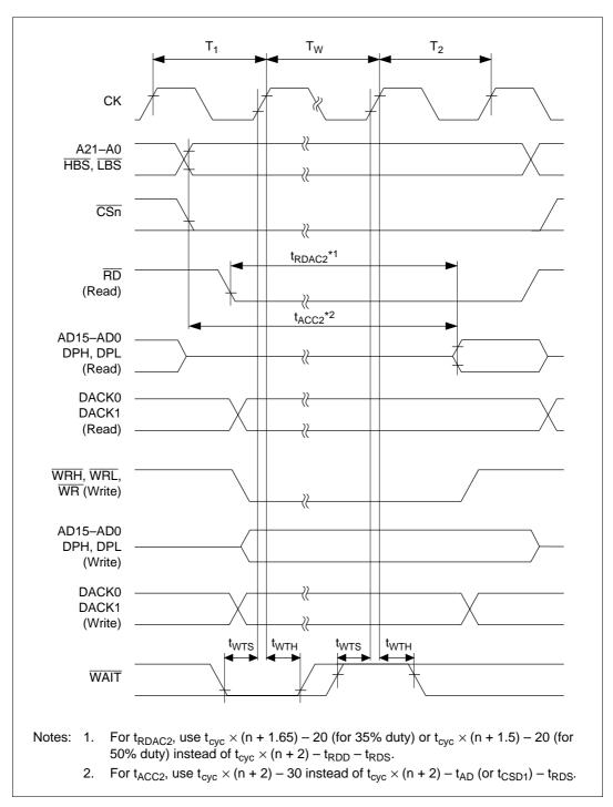
Figure 19.10 Basic Bus Cycle: Two States + Wait State
