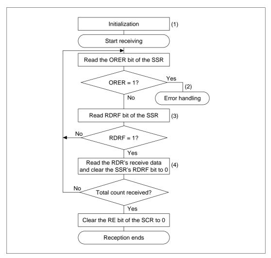
Figure 13.18 Sample Flowchart for Serial Receiving
