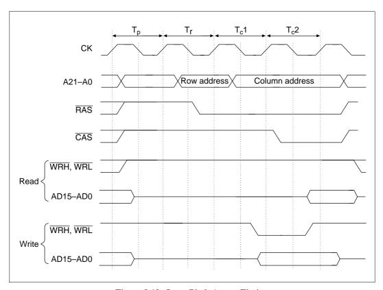
Figure 8.18 Long Pitch Access Timing
