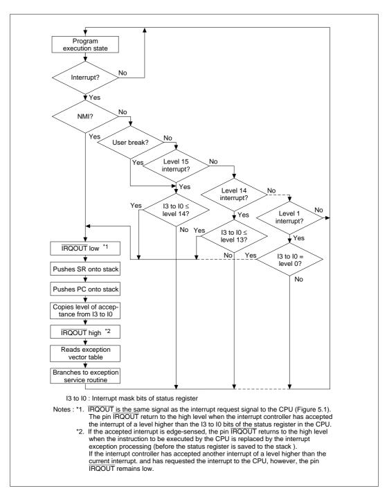
Figure 5.2 Flowchart of Interrupt Operation
