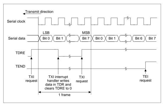
Figure 13.15 Example of SCI Transmit Operation
