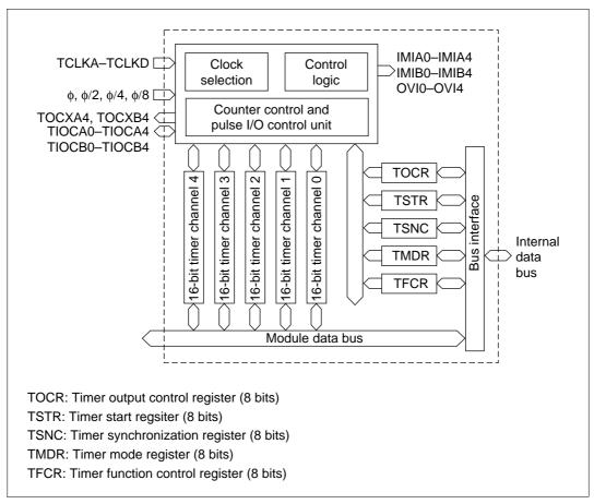
Figure 10.1 ITU Block Diagram
