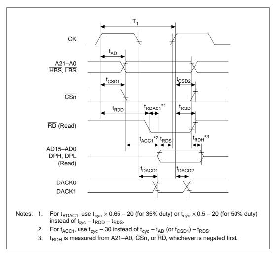
Figure 19.8 Basic Bus Cycle: One-State Access
