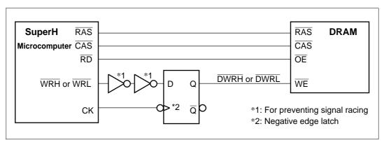
Figure 8.42 Delayed-Write Control Circuit
