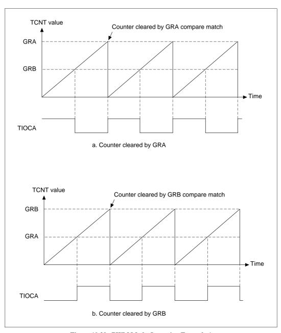
Figure 10.29 PWM Mode Operation Example 1
