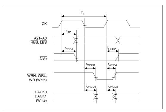
Figure 19.20 DMA Single Transfer/1 State Access Write
