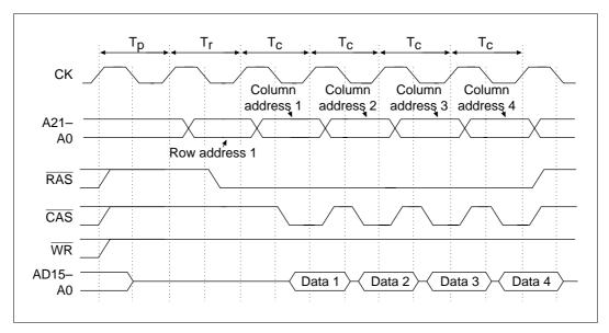
Figure 8.23 Short Pitch High-Speed Page Mode (Read Cycle)
