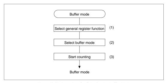
Figure 10.47 Procedure for Selecting the Buffer Mode
