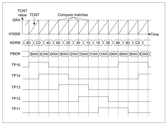
Figure 11.5 TPC Output Example (5-Phase Pulse Output)
