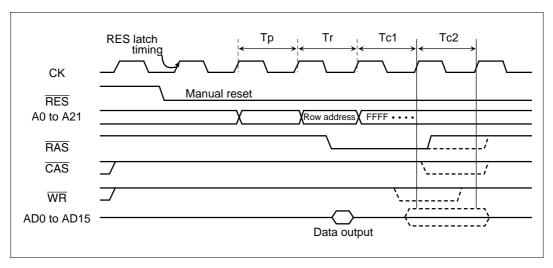
Figure 8.39 Long - pitch Mode Write (2)
