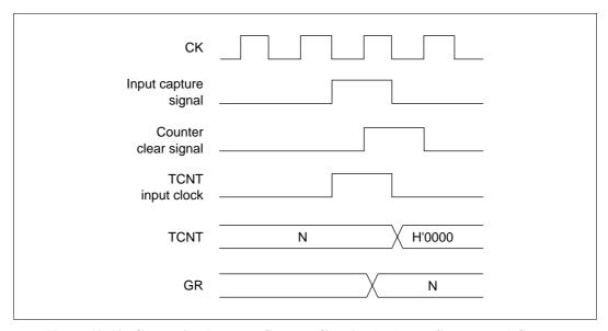
Figure 10.64 Contention between Counter Clearing by Input Capture and Counter Increment
