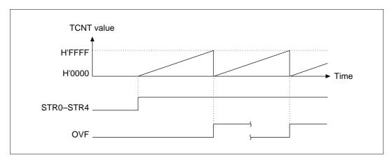
Figure 10.15 Free-Running Counter Operation
