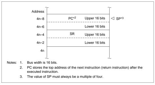
Figure 5.3 Stack after Interrupt Exception Processing
