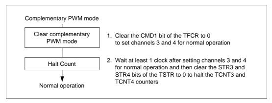
Figure 10.69 Clearing the Complementary PWM Mode
