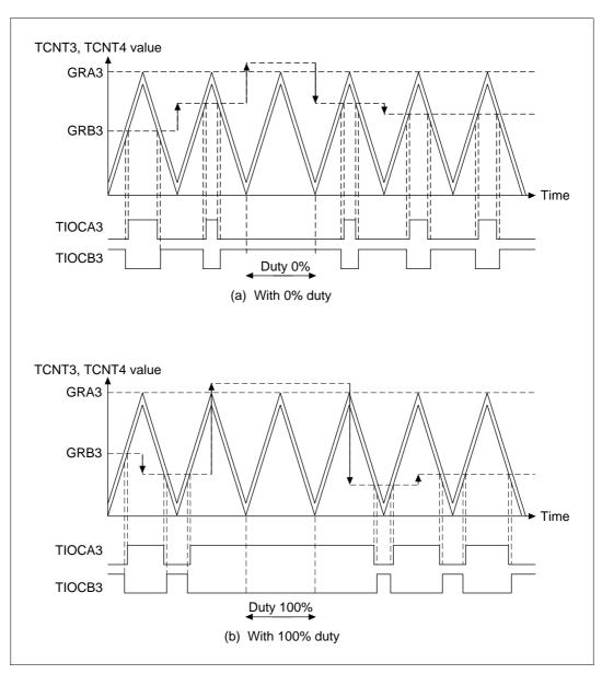
Figure 10.35 Complementary PWM Mode Operation Example 2
