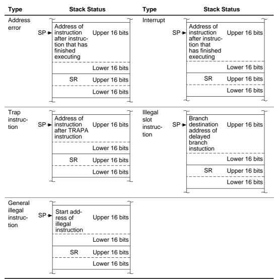
Note: Stack status is based on a bus width of 16 bits.
