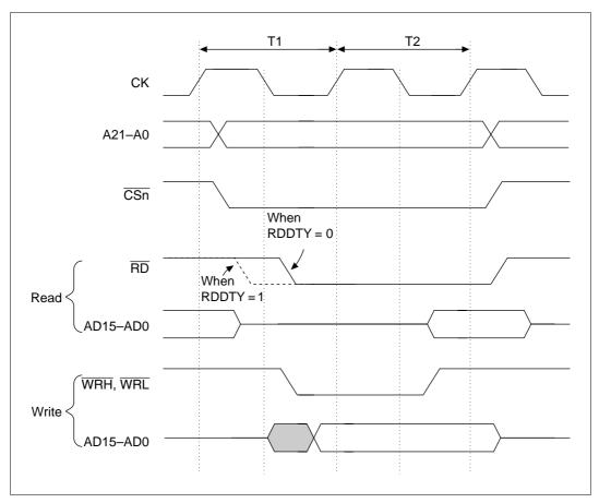
Figure 8.12 Basic Timing of External Memory Space Access (2-state read timing)
