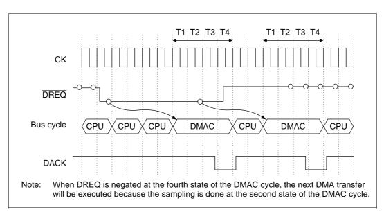
Figure 9.21  $\overline{DREQ}$  Sampling Timing in Cycle Steal Mode (Output with  $\overline{DREQ}$  level detection and DACK active low) (Single address mode, bus cycle = Address/data multiplex I/O bus cycle)
