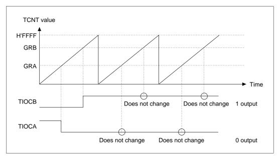
Figure 10.20 Example of 0 Output/1 Output
