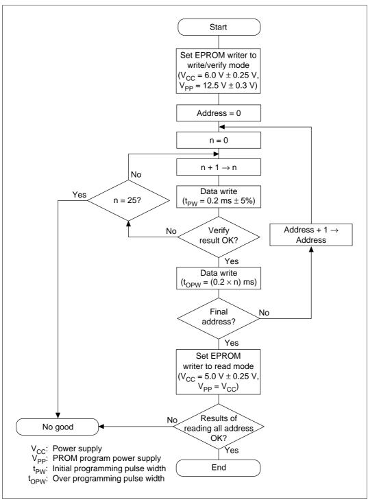
Figure 16.4 Basic Flowchart of High-Speed High-Reliability Programming
