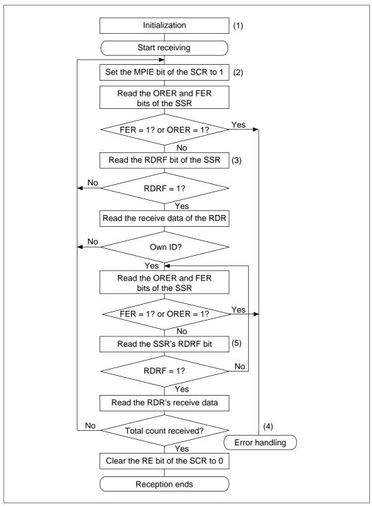
Figure 13.12 Sample Flowchart for Receiving Multiprocessor Serial Data
