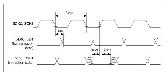
Figure 19.41 SCI I/O Timing (Clocked Synchronization Mode)
