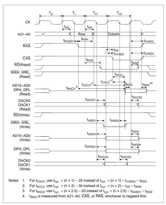
Figure 19.13 DRAM Bus Cycle: (Long Pitch, Normal Mode)
