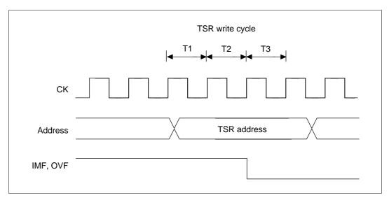
Figure 10.57 Timing of Status Flag Clearing
