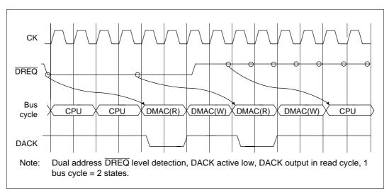
Figure 9.24 DREQ Pin Sampling Timing in Burst Mode
