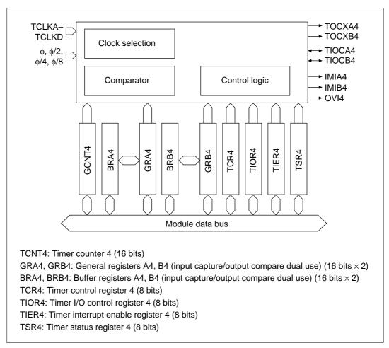
Figure 10.5 Channel 4 Block Diagram
