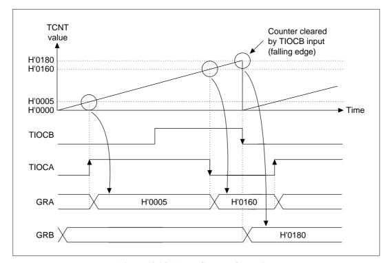
Figure 10.24 Input Capture Operation
