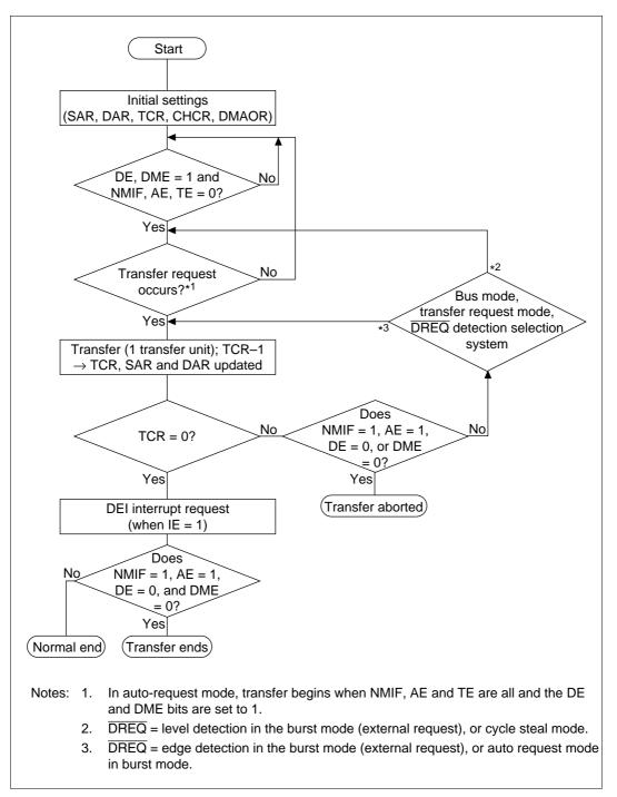
Figure 9.2 DMA Transfer Flowchart
