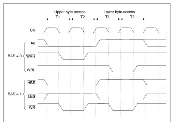
Figure 8.15 Byte Access Control Timing For External Memory Space Access (Write Cycle)
