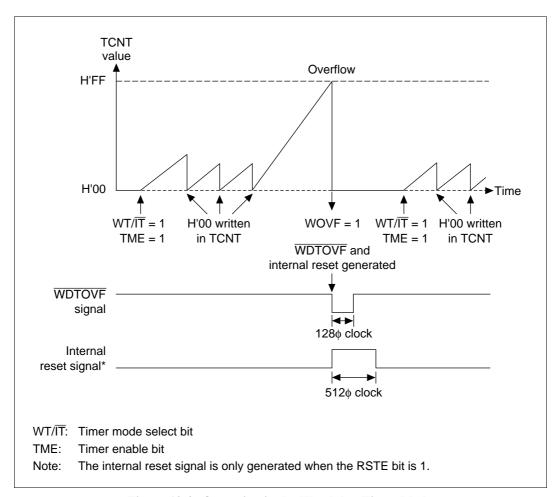
Figure 12.4 Operation in the Watchdog Timer Mode
