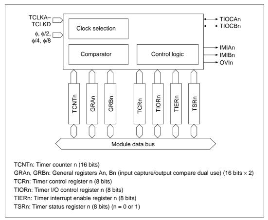
Figure 10.2 Channels 0 and 1 Block Diagram (One Channel Shown)
