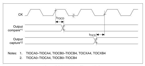
Figure 19.36 ITU Input/Output Timing
