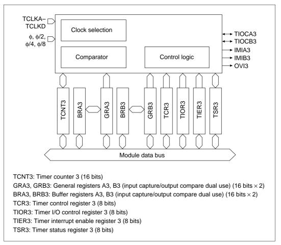
Figure 10.4 Channels 3 Block Diagram
