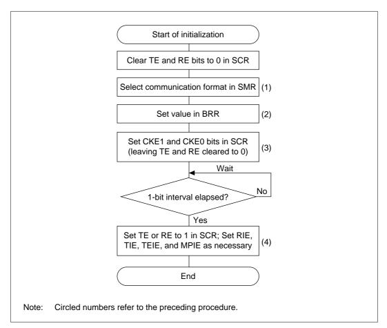
Figure 13.4 Sample Flowchart for SCI Initialization
