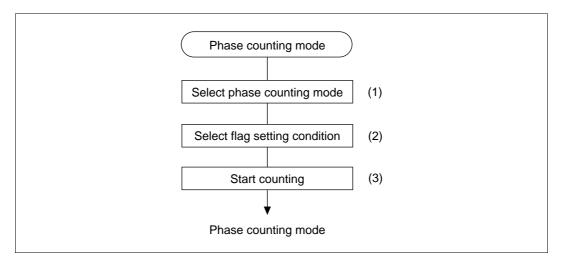
Figure 10.42 Procedure for Selecting the Phase Counting Mode
