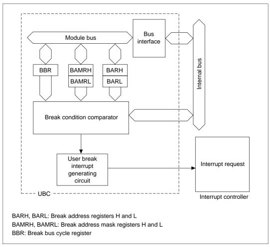
Figure 6.1 Block Diagram of the User Break Controller
