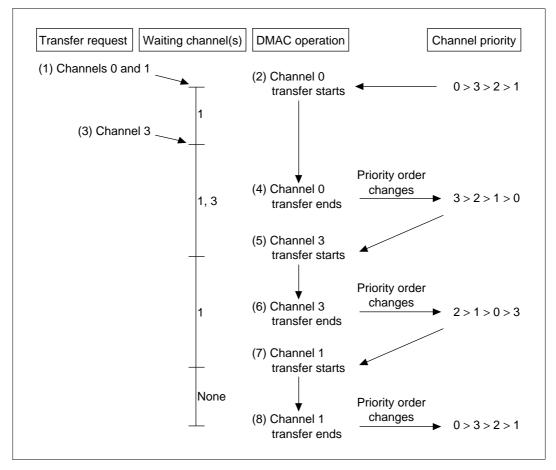
Figure 9.4 Changes in Channel Priority in Round-Robin Mode
