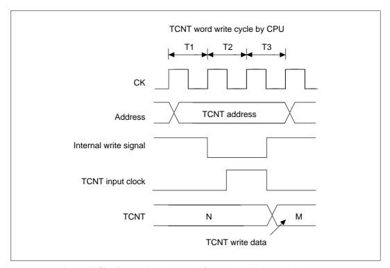
Figure 10.59 Contention between TCNT Word Write and Increment
