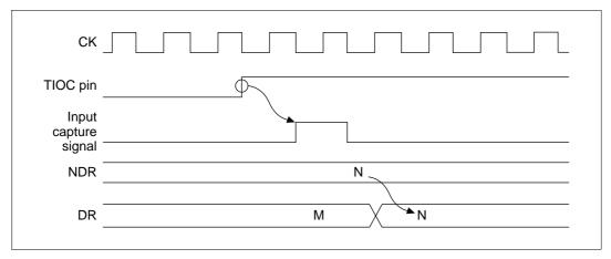
Figure 11.8 TPC Output by Input Capture
