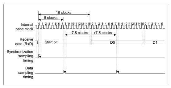
Figure 13.21 Receive Data Sampling Timing in Asynchronous Mode
