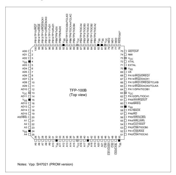
Figure 1.2 Pin Arrangement
