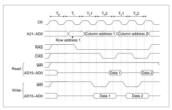
Figure 8.26 Long Pitch High-Speed Page Mode (Read/Write Cycle)
