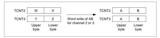
Figure 10.68 Word Write to Channel 2 or Word Write to Channel 3
