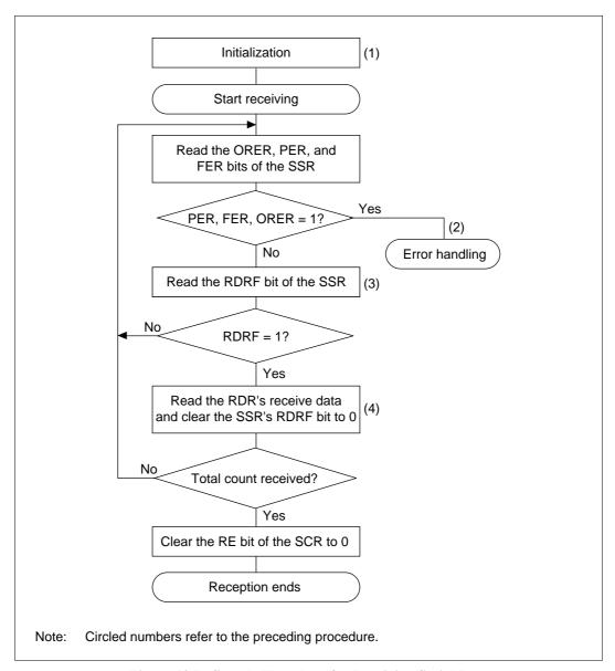
Figure 13.7 Sample Flowchart for Receiving Serial Data
