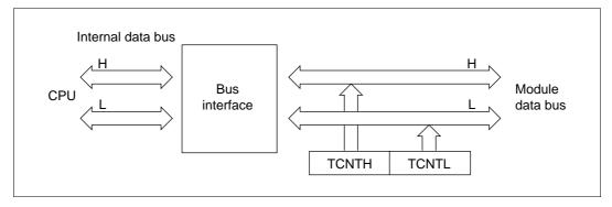
Figure 10.10 Accessing TCNT (TCNT-CPU (upper byte))
