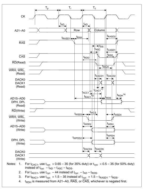
Figure 19.24 DRAM Bus Cycle (Short Pitch, Normal Mode)
