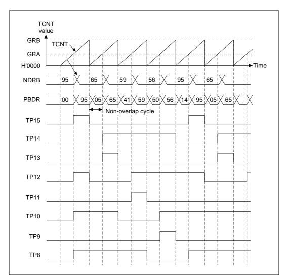
Figure 11.7 Non-Overlap Output Example (Four-Phase Complementary Output)
