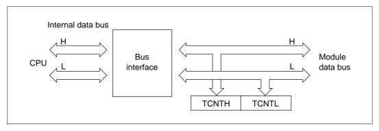
Figure 10.6 Accessing TCNT (CPU-TCNT (word))
