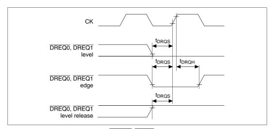
Figure 19.34 DREQ0, DREQ1 Input Timing (1)
