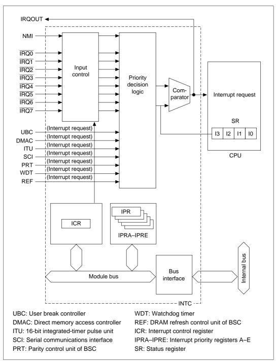
Figure 5.1 Block Diagram of the Interrupt Controller
