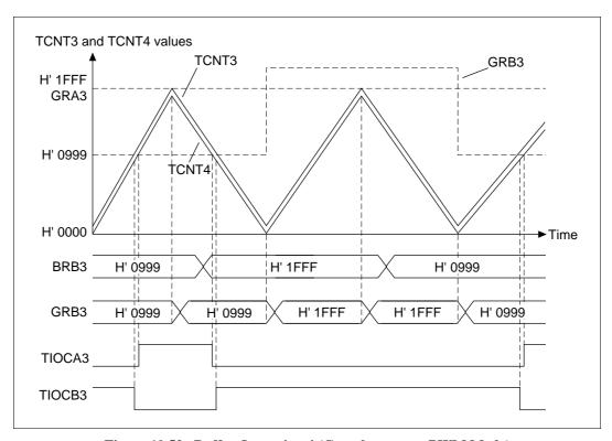
Figure 10.52 Buffer Operation 4 (Complementary PWM Mode)
