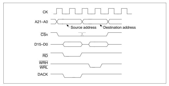
Figure 9.9 DMA Transfer Timing in the Dual Address Mode (External memory space to external memory space transfer with DACK output in the read cycle)
