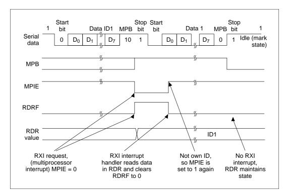
Figure 13.13 shows an example of SCI receive operation using a multiprocessor format.
