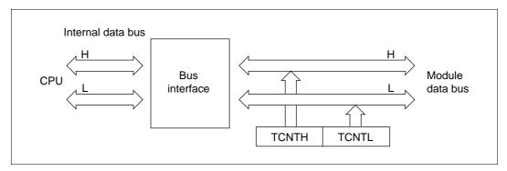
Figure 10.11 Accessing TCNT (TCNT-CPU (lower byte))
