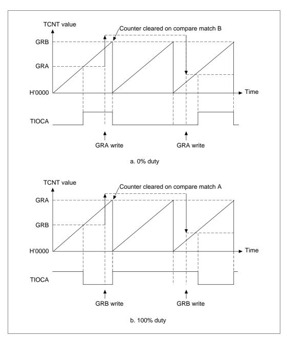
Figure 10.30 PWM Mode Operation Example 2
