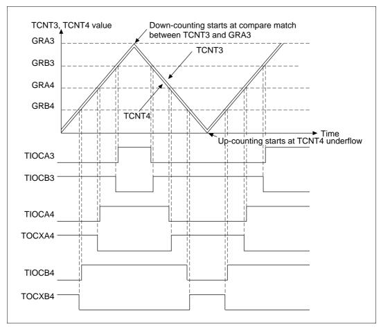
Figure 10.34 Complementary PWM Mode Operation Example 1
