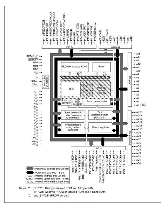
Figure 1.1 Block Diagram
