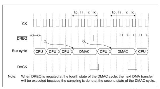
Figure 9.19  $\overline{DREQ}$  Sampling Timing in Cycle Steal Mode (Output with  $\overline{DREQ}$  level detection and DACK active low) (Single address mode, bus cycle = DRAM bus cycle (long pitch normal mode))
