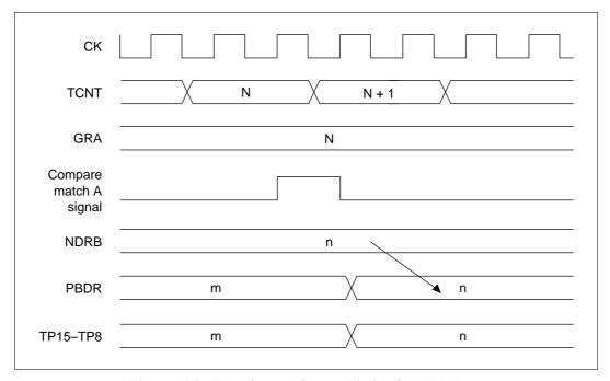
Figure 11.3 Transfer and Output Timing for NDR Data
