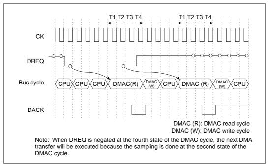
Figure 9.22  $\overline{DREQ}$  Sampling Timing in Cycle Steal Mode (Output with  $\overline{DREQ}$  level detection and DACK active low) (Dual address mode, bus cycle = Address/data multiplex I/O bus cycle)
