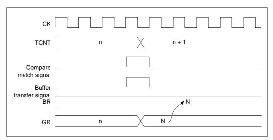
Figure 10.49 Compare Match Timing Example for Buffer Operation
