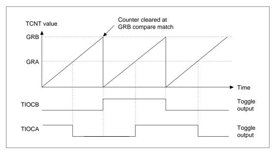
Figure 10.21 Example of Toggle Output
