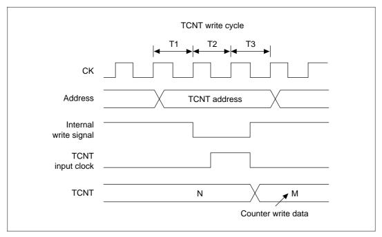
Figure 12.8 Contention between TCNT Write and Increment
