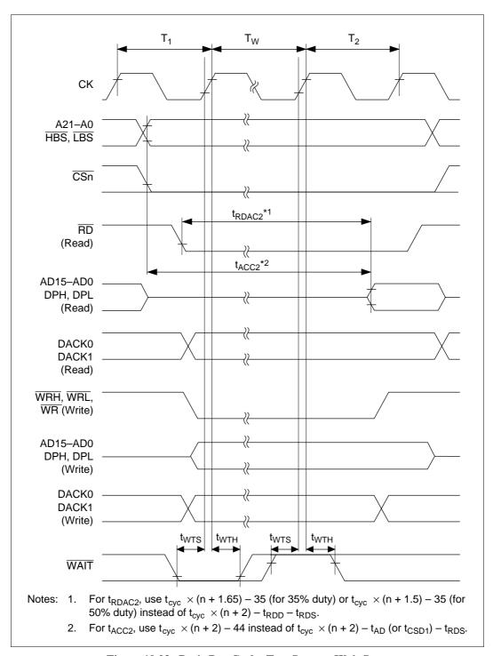
Figure 19.23 Basic Bus Cycle: Two States + Wait State
