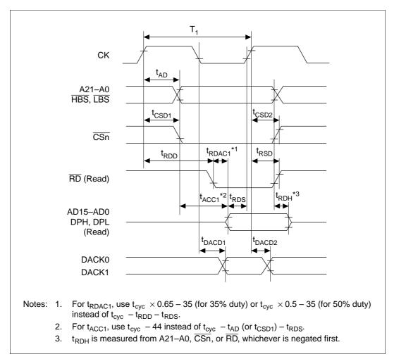
Figure 19.21 Basic Bus Cycle: One-State Access
