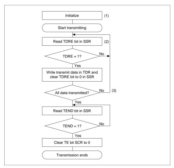
Figure 13.17 Sample Flowchart for Serial Transmitting
