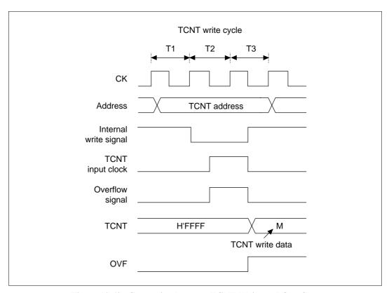
Figure 10.62 Contention between TCNT Write and Overflow
