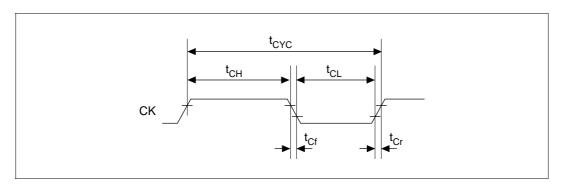
Figure 19.2 System Clock Timing
