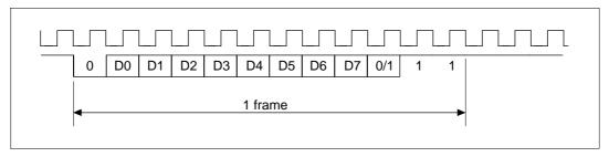
Figure 13.3 Phase Relationship Between Output Clock and Serial Data (asynchronous mode)
