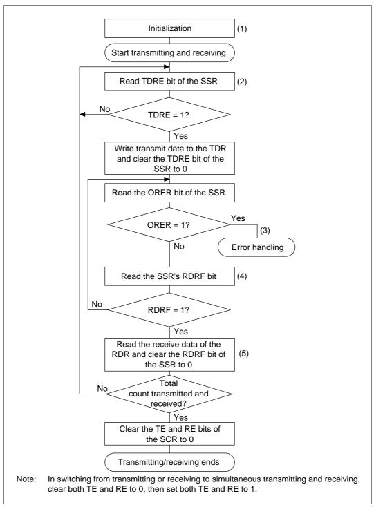
Figure 13.20 Sample Flowchart for Serial Transmitting
