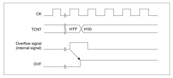
Figure 12.6 Timing of Setting the OVF
