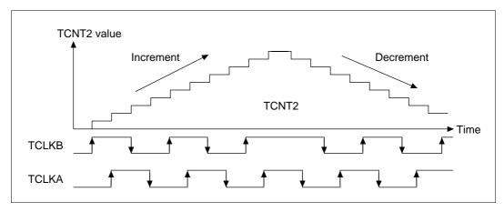
Figure 10.43 Phase Counting Mode Operation
