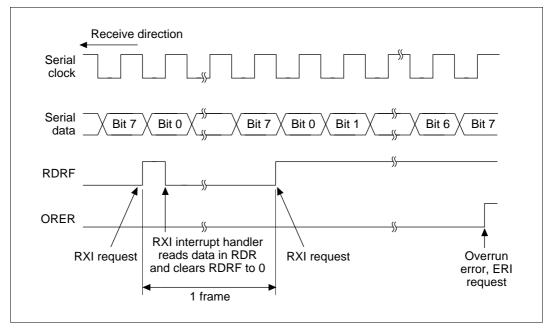
Figure 13.19 Example of SCI Receive Operation
