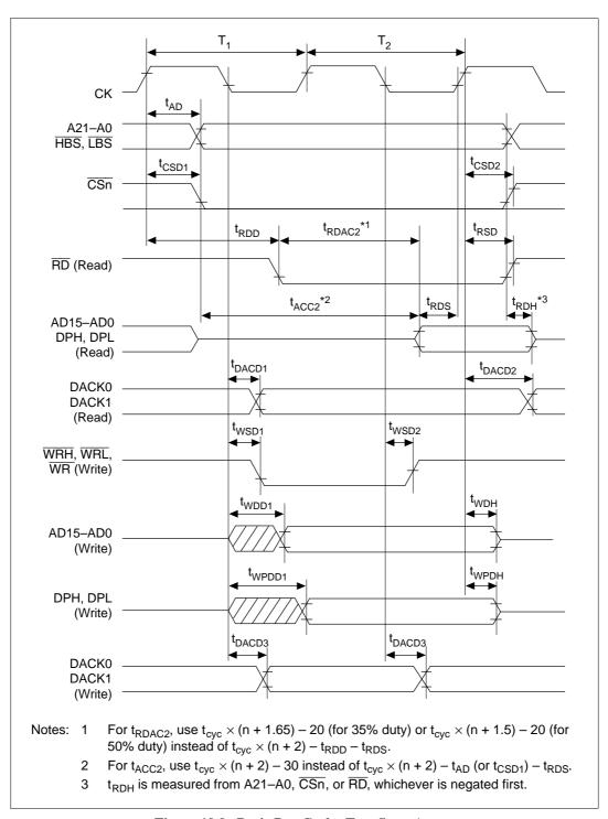
Figure 19.9 Basic Bus Cycle: Two-State Access
