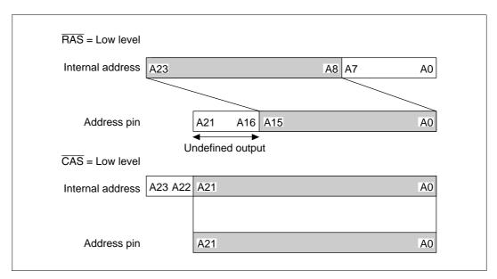
Figure 8.16 Address Multiplexing States (8-bit shift)
