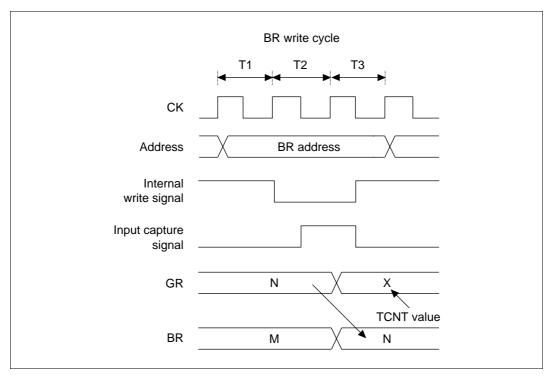
Figure 10.66 Contention between BR Write and Input Capture
