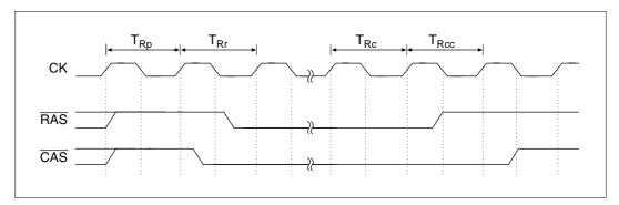
Figure 8.31 Output Timing of Self-Refresh Signal
