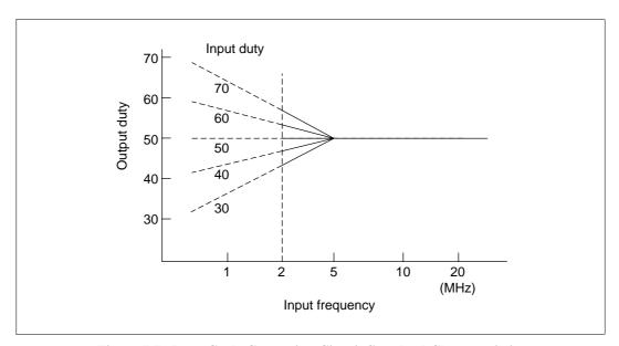
Figure 7.7 Duty Cycle Correction Circuit Standard Characteristics
