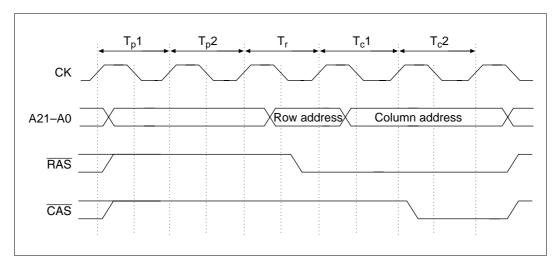
Figure 8.19 Precharge Timing (Long Pitch)
