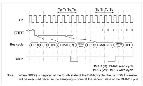
Figure 9.20  $\overline{DREQ}$  Sampling Timing in Cycle Steal Mode (Output with  $\overline{DREQ}$  level detection and DACK active low) (Dual address mode, bus cycle = DRAM bus cycle (long pitch normal mode))
