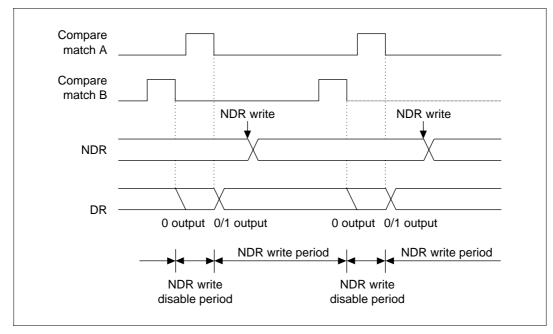
Figure 11.10 Non-Overlap Operation and NDR Write Timing
