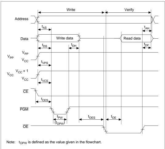
Figure 16.5 Write/Verify Timing
