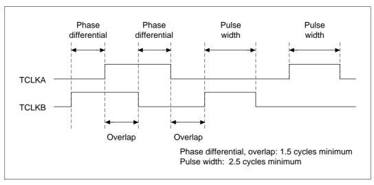
Figure 10.44 Phase Differentials, Overlap and Pulse Width in the Phase Counting Mode
