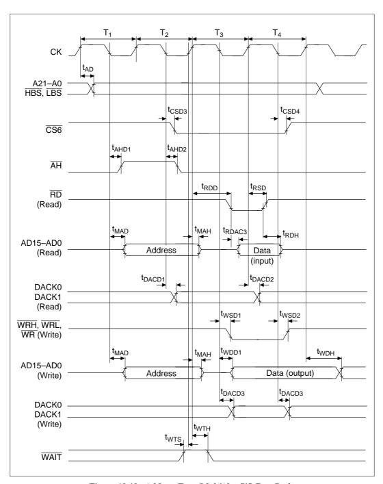
Figure 19.19 Address/Data Multiplex I/O Bus Cycle
