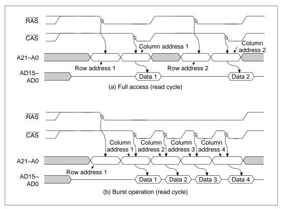
Figure 8.22 Full Access and Burst Operation
