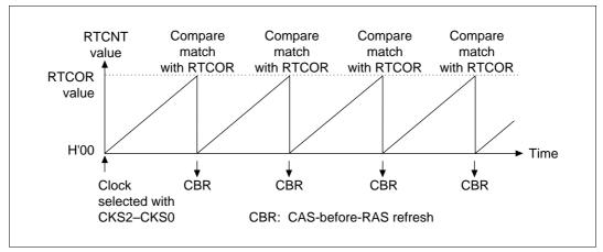
Figure 8.29 Refresh Timer Counter (RTCNT) Operation
