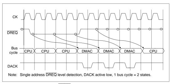
Figure 9.23 DREQ Pin Sampling Timing in Burst Mode
