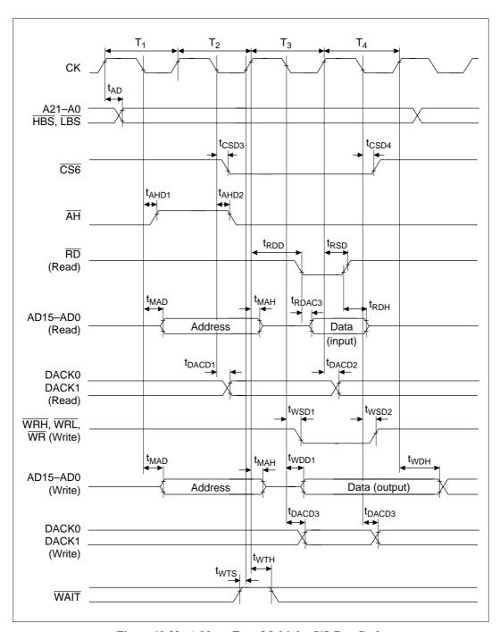
Figure 19.32 Address/Data Multiplex I/O Bus Cycle
