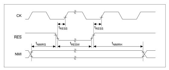
Figure 19.4 Reset Input Timing
