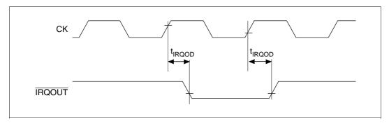
Figure 19.6 Interrupt Signal Output Timing
