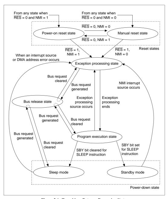
Figure 2.6 Transitions Between Processing States
