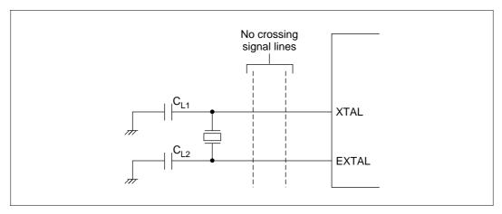
Figure 7.6 Precaution on Oscillator Circuit Board Design
