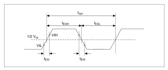
Figure 7.5 Input Clock Waveform
