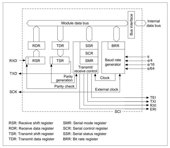
Figure 13.1 SCI Block Diagram
