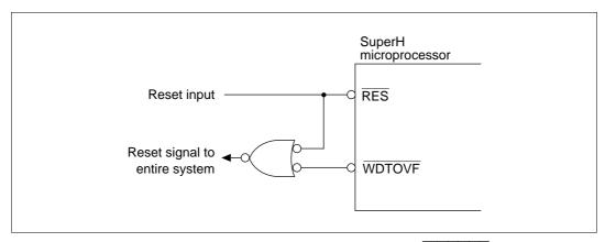
Figure 12.9 Example of a System Reset Circuit with a WDTOVF Signal
