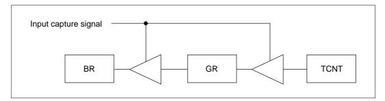
Figure 10.46 Input Capture Buffer Operation
