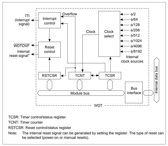
Figure 12.1 WDT Block Diagram
