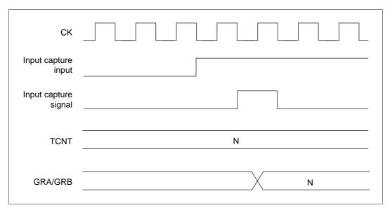
Figure 10.25 Input Capture Signal Timing
