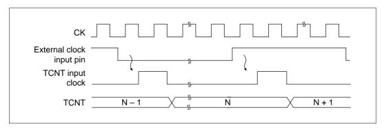
Figure 10.18 Count Timing for External Clock Sources
