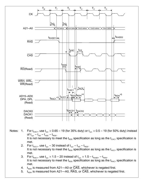
Figure 19.12 (a) DRAM Bus Cycle (Short-Pitch, High-Speed Page Mode: Read)
