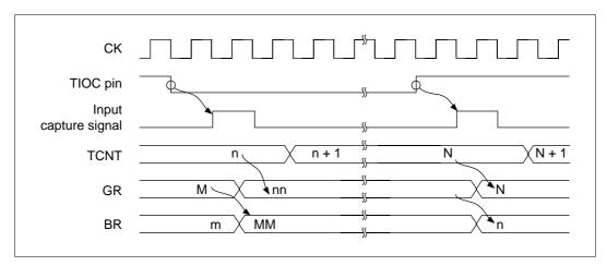
Figure 10.51 Input Capture Timing Example for Buffer Operation
