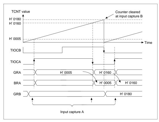
Figure 10.50 Buffer Mode Operation Example 2 (Input Capture Register)
