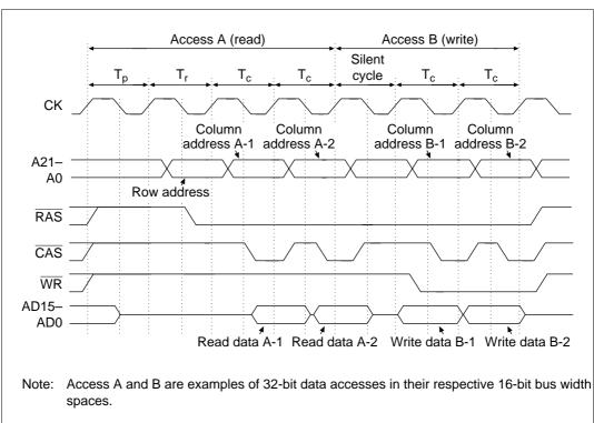
Figure 8.25 Short Pitch High-Speed Page Mode (When read and write cycle continues with
