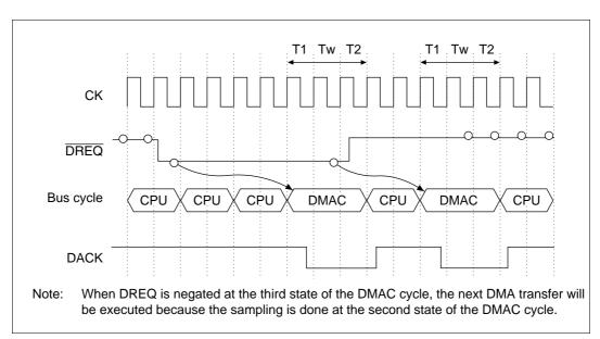
Figure 9.17  $\overline{DREQ}$  Sampling Timing in Cycle Steal Mode (Output with  $\overline{DREQ}$  level detection and DACK active low) (Single address mode, bus cycle = 2 states + 1 wait state)
