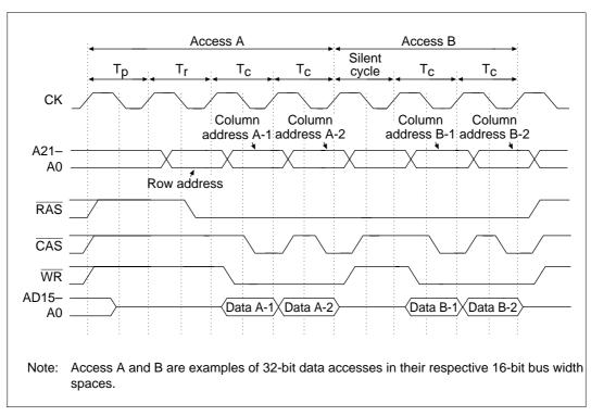
Figure 8.24 Short Pitch High-Speed Page Mode (Write Cycle)
