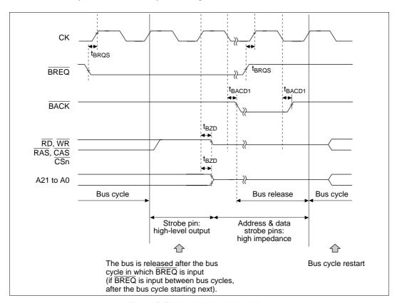
Figure 8.47 Bus Release Procedure
