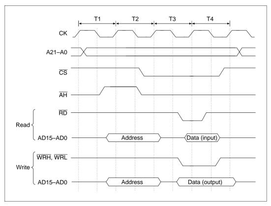
Figure 8.32 Access Timing For Address/Data Multiplexed I/O Space
